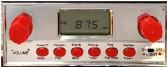
Press the Power
